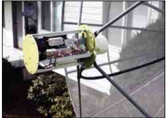
Fig 5 —This photo shows W7LHL's 10-GHz equipment that is mounted at the feed for the parabolic dish shown in Fig 4. A DB6NT transverter, along with an MKU-101B receive preamplifier (0.8-dB noise figure), a driver amplifier and an MKU-102XL output amplifier (all from Kuhne Electronic) are at the feed. A waveguide TR switch minimizes losses at the feed horn. A frequency-reference signal comes from the shack on a coaxial cable to phase-lock the crystal oscillator in the transverter.
